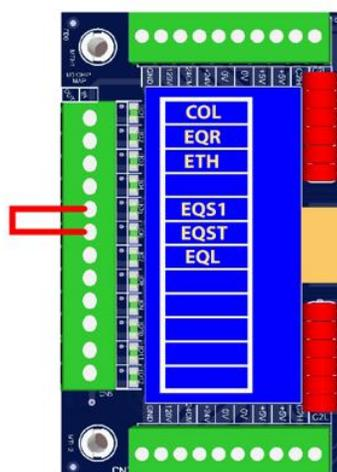
Figure 2: Typical I/O Expansion Board
